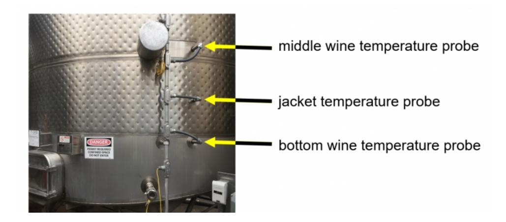
This allows the cascade routine to refill (or pulse), fresh coolant into the jacket coolant when the temperature difference from coolant to content (i.e. wine) is no longer enough to cool the content effectively. This method is currently in place at Beringer Winery. Future work will benchmark this method against the other two methods described above.
