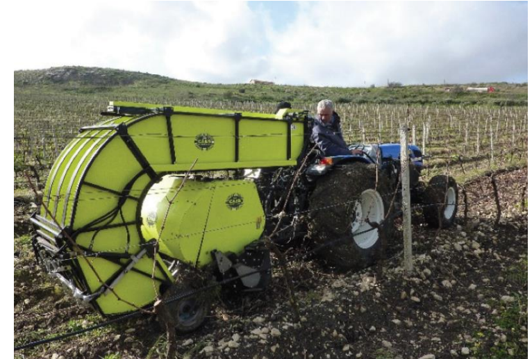
Figure: CAEB Baler at work in the vineyard. Creates bales of prunings.
