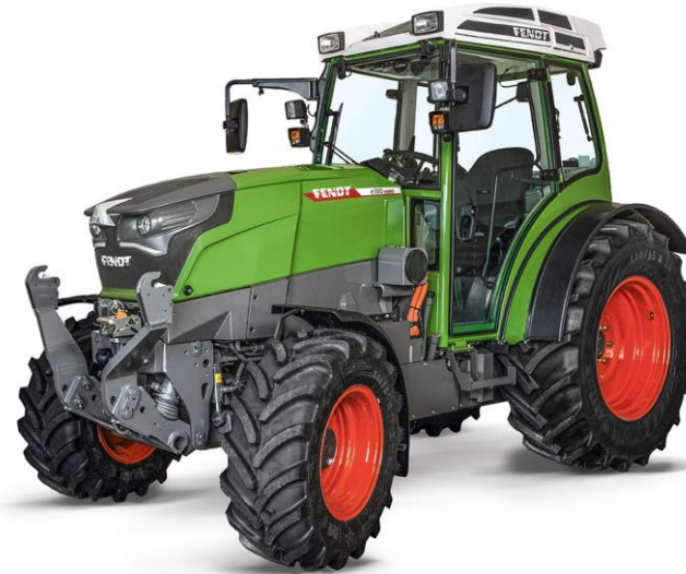
Figure: Fendt e100 tractor prototype as presented at Agritechnica 2017 (50 kW, 100 kWh battery)
